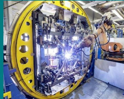
workstations for the welding phases. It's then the phase of the cathodic dip-paint coating (KTL), with subsequent drying at 90° and 220° and sealing to prevent corrosion. The bodywork is then sent to the Neu-Ulm plant for paneling and painting.
