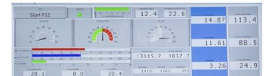
During the demonstration test, the central eCitaro energy management system was connected to a computer in order to display a screen with all consumption data, from moment to moment (see image on the side). Next to the speed indicator (on the left) is displayed the immediate percentage of power consumed (in red) or recovered (in green), while on the right is displayed the
