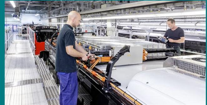
When it is sent back to Mannheim, the assembly phase begins. Components are placed on the roof and the high voltage cables (orange) are laid from a raised position. Then the windows are glued, the platform is assembled, the air tanks and air conditioning pipes are installed. Then it's the
